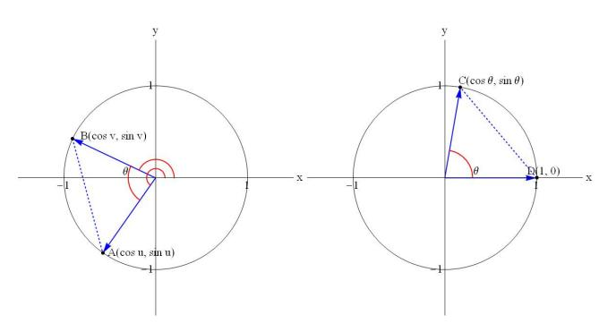
The sketch on the left can be rotated so the angle  $\theta$  is in standard position (initial side along the x axis). This gives the sketch on the right.
