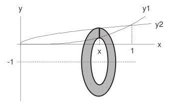
I have drawn my sketch slightly more general than it needs to be. The curves are  $y_1 = x^3$  and  $y_2 = \sqrt{x}$ . The region being rotated is the area between the two curves. As x moves between 0 and 1, the small line in the region will sweep out the entire region. This tells us that we should integrate with respect to x, and we should have integration limits of 0 and 1.
